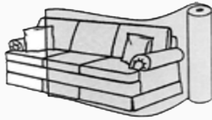
Fabric application as applied Railroaded during the upholstery process.
