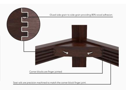
The connection of the seat rails is the foundation of a chair's strength. Our Lock Block construction creates the most stable chair base, even under extreme stress, making the entire chair exponentially stronger. Lock Block Construction also more than doubles the glue bond surface allowing for greater adhesion. The seat frame will not flex out of its intended shape and will transfer stress to other points of the chair.
